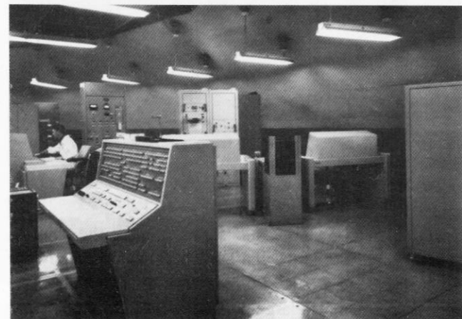
Operational shot of Launch Operations. The console for the Univac Athena computer is in the foreground with the launch consoles in the background. (Photograph courtesy of www.chromehooves.net )
